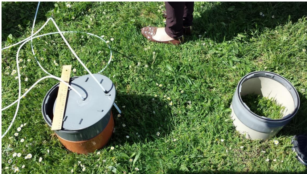
The IAEA in-house made soil chambers.
