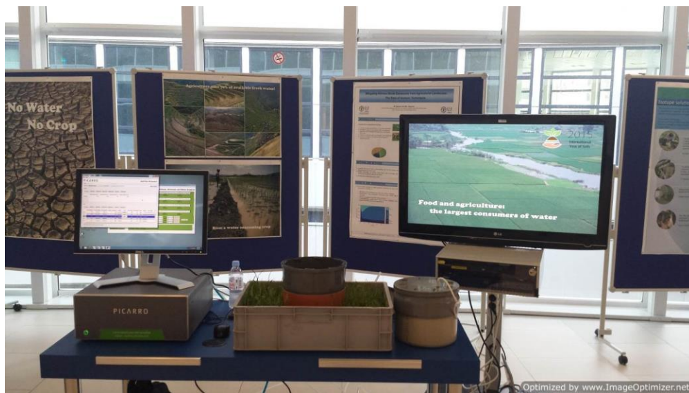
The Picarro G2508, a simultaneous five species concentration instrument for measuring CO_2 , CH_4 , N_2O , NH_3 and H_2O , at the Global Soil week exhibition at the IAEA headquarters in Vienna.
